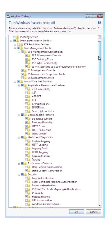
The Microsoft web server for Vista is IIS 7.0, which is provided as part of the standard distribution. A default installation of IIS 7.0 does not support running a CGI application such as Mascot. From the Control Panel, choose 'Programs and Features'. Choose 'Turn Windows features on or off'. Expand the node for Internet Information Services and ensure that all the checkboxes shown below are checked, in addition to any default selections. Then, choose OK.
