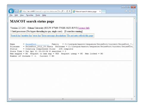
If an error occurs, use the links to the monitor log and the error log to investigate the cause. If all is well, you will see the following messages displayed on the status line for SwissProt:
