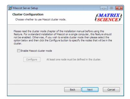
If you have a multi-CPU licence, you can configure Mascot for execution on a networked cluster. If you intend to do this, refer to Chapter 11 for further details before proceeding. If you are installing Mascot on a single multiprocessor server, leave the Enable cluster mode checkbox clear.
