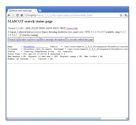
If an error occurs, use the links to the monitor log and the error log to investigate the cause. If all is well, you will see the following messages displayed on the status line for SwissProt:
