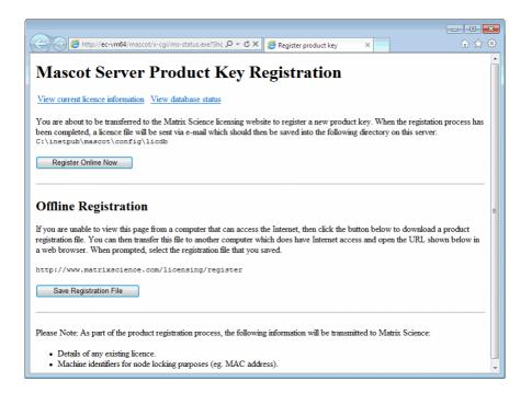
A product key is required and must be registered online. The licence file will be returned by email and must be saved to the specified location on the Mascot server. If the Mascot server cannot connect to the Internet, a file containing registration information can be saved and copied to a system with Internet access for submission.
