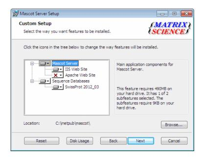
If IIS is installed and functional, the default selections will be as shown above, with IIS being configured automatically. If you don't have IIS installed, the Apache option will be selected instead. A test for whether Apache or some other web server is actually installed comes later.
