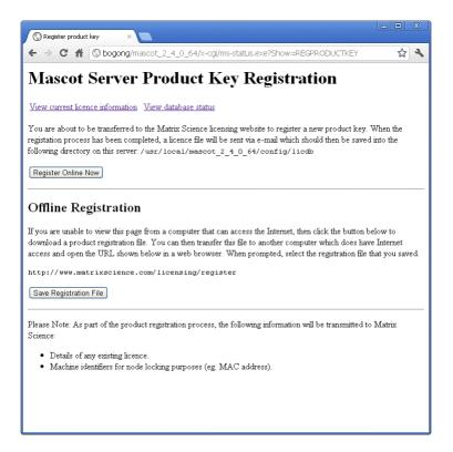
A product key is required and must be registered online. The licence file will be returned by email and must be saved to the specified location on the Mascot server. If the Mascot server cannot connect to the Internet, a file containing registration information can be saved and copied to a system with Internet access for submission.
