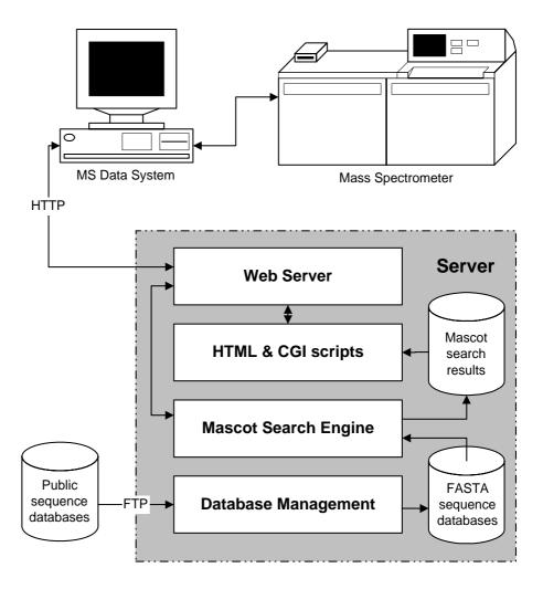
digest of the results) to the client. Links to additional CGI scripts provide more detailed views of the results.
