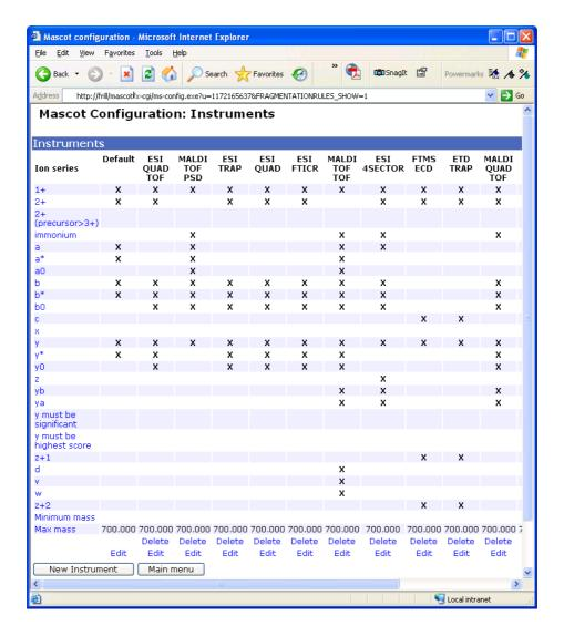
The INSTRUMENT search parameter is used to select the set of ion series used for scoring MS/MS matches.
